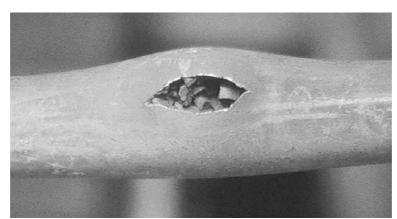
Ballooning and relocalisation of the fuel in the ballooned area during the ICL#2 integral test carried out at the Argonne National Laboratory (USA)
